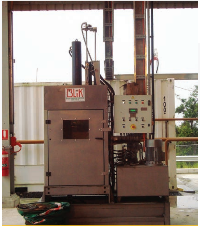
The drum crusher at the Hides Waste Management Facility
