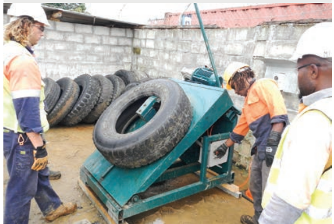
A used tire being prepared for cutting with the Ecoflex system
